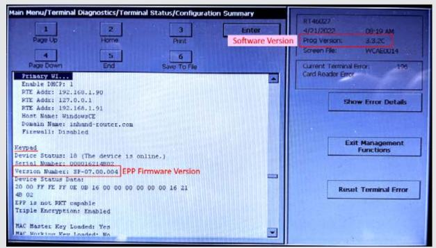
The Version Number must show "414-0737" at a minimum. Any other values for the Version number means that the keypad will need replaced.
