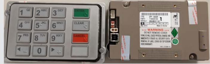
EPP-X1 – Additional paneling that prevents easy access to back of keypad, external pressure switches.
