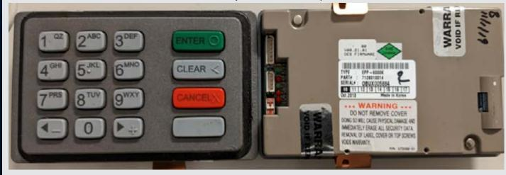
8000R – buttons are more flat with body and external pressure switches.
